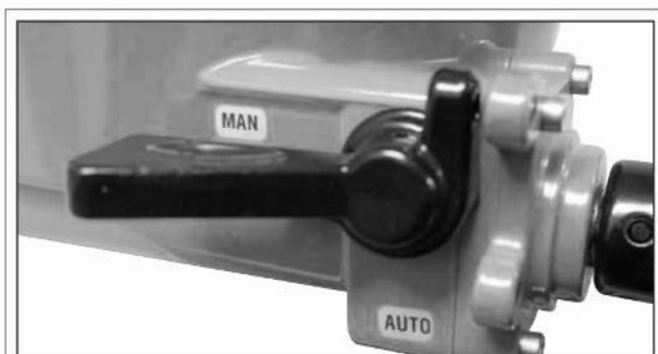
Fig.11 Particular of the "S" selector in "MAN" position.
